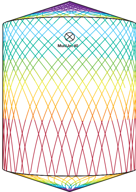
D5m H6m, Toftejorg MultiJet 40, 4 x ø6 mm, 100% Time = 4.3 min., Water consumption = 887 l (234 gallon)
