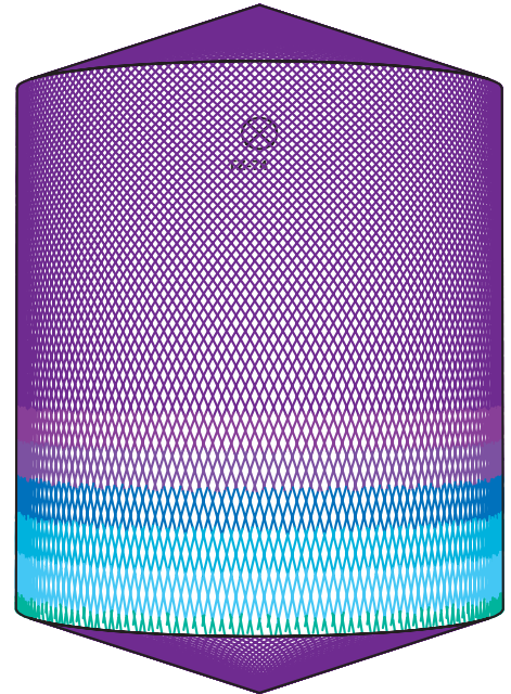
D5m H6m, Toftejorg TZ-74 Self Cleaning version, 4 x ø7 mm, 0% Time = 15.3 min., Water consumption = 4853 l (1282 gallon)
